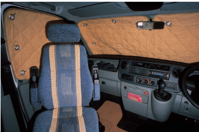
We prefer curtains to the suction cup-equipped insulating pads provided for cab blackout.
