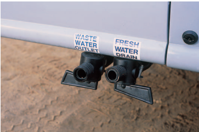
Clearly marked, but fiddly to use, drain valves serve rather small fresh and waste water tanks.
