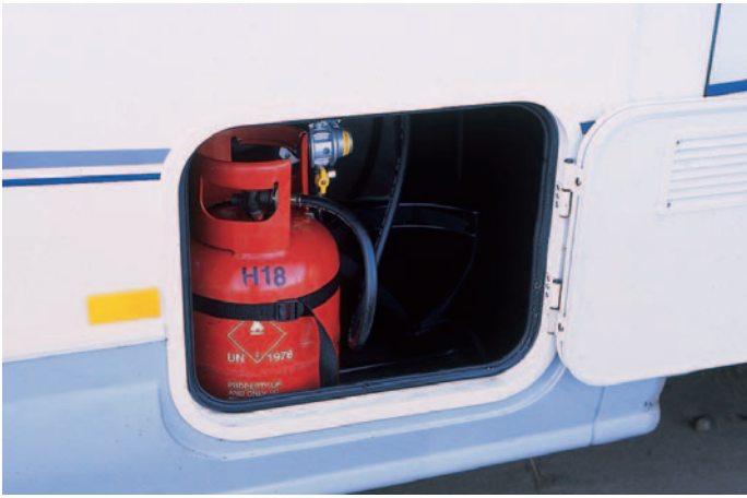
The gas locker accommodates two 6kg/7kg cylinders but a bigger door would be nice.
